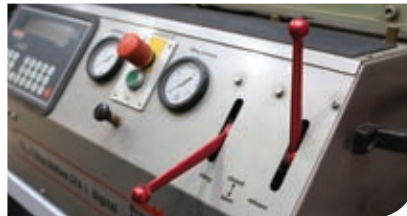
CO2 Extinguisher Filling Machine
