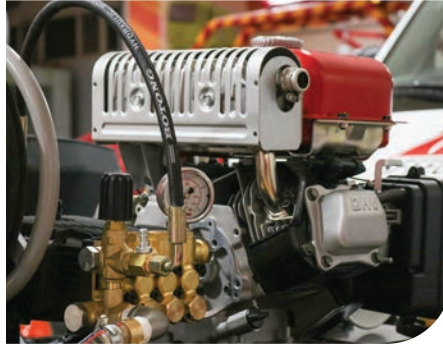
High pressure Pump Linhai Brand Gasoline Engine Model: SPE 175 (2 Units)
